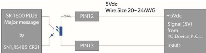
Figure 9-3. Application diagram of dry contact pin12~13(Major)
