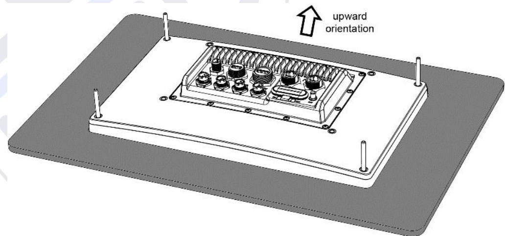
3. Fasten the brackets (supplied with device) with threaded studs and thumb nuts. The nuts shall be tightened carefully by hand to prevent them from loosening due to vibration, while making sure not to damage the Q Display from overtightening.
