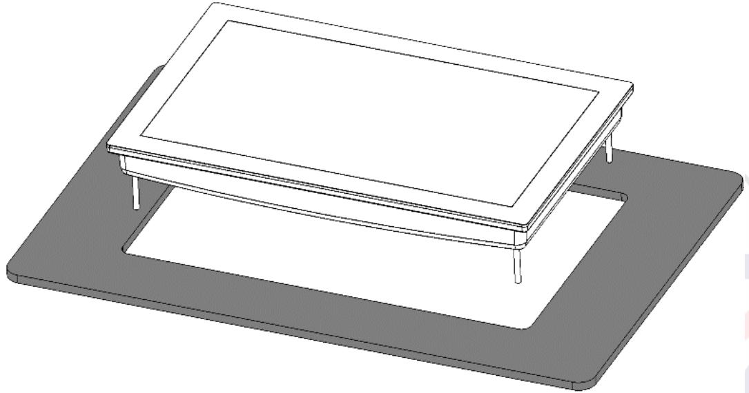
2. After inserting the Q display, check that it is properly in place considering the orientation and that the seam around the screen edge is properly sealed on all sides.
