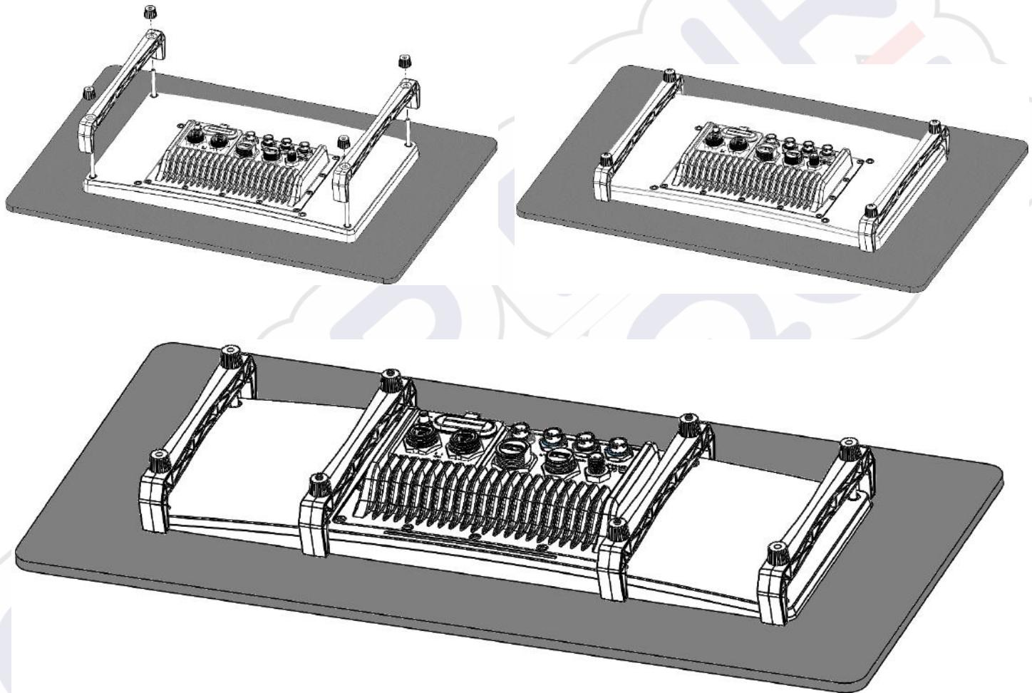
Note that the Q Display 210D (Dual 10") requires 4 brackets (supplied with device).
