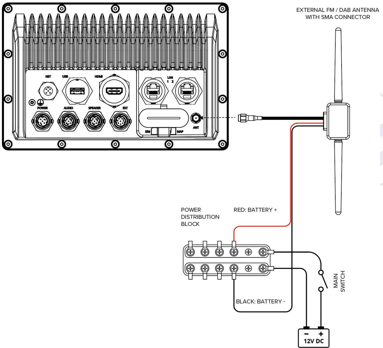
Connect FM/DAB antenna (provided separately) to the Q Display ANT connector. You can use FM/DAB antenna with SMA connector, or you can use SMA male to DIN female adapter cable and connect any FM/DAB antenna with DIN male connector to the adapter cable.
